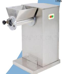
This machine is used mainly in such trades as pharmacy, chemical industry, food, pottery and plastics extensively, making moist powder material particle. Make cylinder swing reciprocatly, extruding material from screen mesh for granulation. It also can be used for crushing the agglomerate materials into small granules directly.
