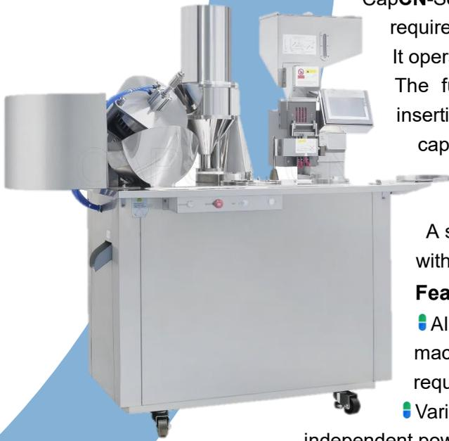
CapCN-Semi vertical type results in faster production, meeting G.M.P. requirements, more accurate filling, a safer operation, simple maintenance. It operate without noise and cleaning is simple.
