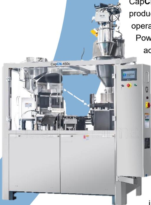
CapCN-450C automatic capsule filler processes the products for optimal productivity up to 7500 capsules per minutes, featuring low-maintenance operation, minimal downtime, and overall dependable production.
