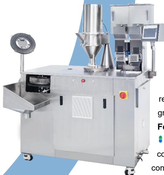
This machine adopts programming control system, touch panel operation, stepless frequency conversion speed regulation, pneumatic joint control, and electronic automatic counting device, which can automatically complete the capsule positioning, separation, filling, locking and other actions.
