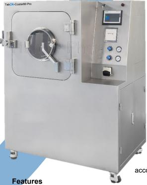
The efficient coating machine is experimental equipment for special use widely applied in Chinese and western tablets, pills and the like for carrying out water phase and organic film coating. This equipment is manufactured in strict accordance with the requirements of pharmaceuticals industry association "GMP", and all shells, coating rollers, heat fans, exhaust fans, spraying devices, and all components in contact with drugs are produced by stainless steel materials.
