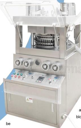
The machine is a double-pressing automatically revolving piece-pressing machine which could make grain be pressed to be round piece ,be carved characters ,special shapes and double color piece prescription .It is mainly used in manufacturing piece prescription for pharmaceutical industry enterprises like chemical industry ,foods, electronics .
