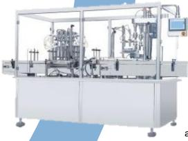
LiqCN-8 Series Piston Bottle Filling Machine is design to provide flexible filling capability for all your applications from light liquids to heavy creams and gels. Automatic models are available in three dispensing ranges: 30-100mL (up to 80 cpm), 100-500mL (up to 60 cpm) and 500-1,000mL (up to 50 cpm) with little additional change parts.
