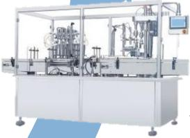
liqCN-4A Series Piston Bottle Filling Machine is design to provide flexible filling capability for all your applications from light liquids to heavy creams and gels. Automatic models are available in three dispensing ranges: 0-100mL (up to 40 cpm), 100-500mL (up to 30 cpm) and 500-1,000mL (up to 25 cpm) with little additional change parts.
