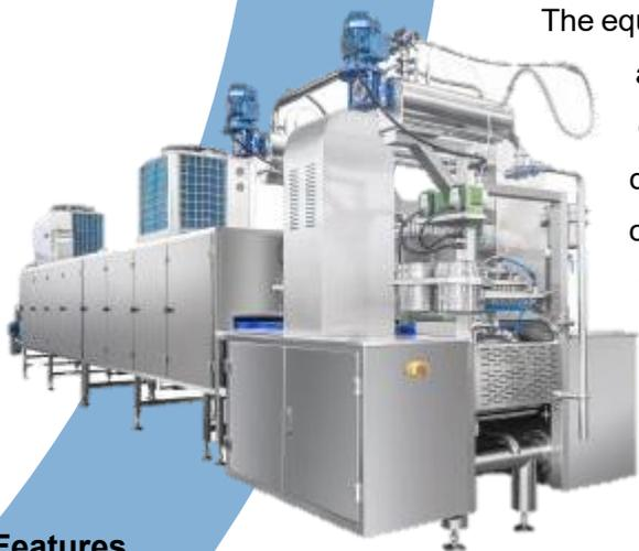
The equipment for making gelatin jelly candy comprises a cooking section, a depositing section, and a cooling section. The GD150 line uses one-row molds and can produce 100-150kg of candy per hour, depending on the weight of the pieces. The candy's shape can be customized to suit the customer's needs, and various designs are available. The candy can be made in single or double colors, with left-right or up-down patterns. Examples of the final product are provided in the photos below.
